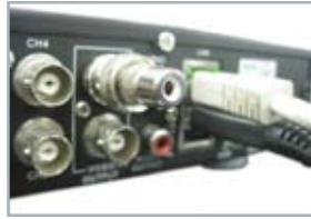
Plug RCA cable to BNC
